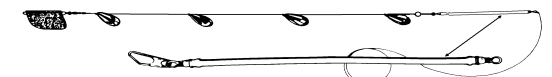
Snubbers are attached between the troll and the leader to the lure and absorb the shock of hard strikes. They are available in light, medium or heavy-duty sizes to work with the pound test leader you select.
